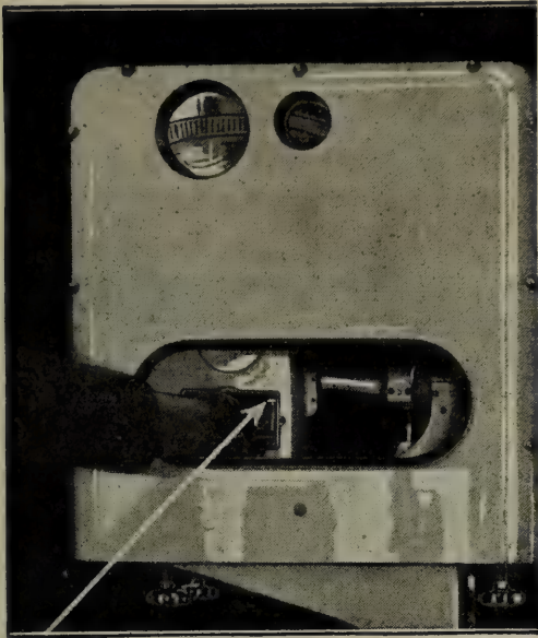
Fig. 105. Adjusting Movement of Pointer By Means of Screw B.
